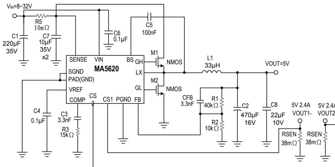
$$V_{OUT} = V_{FB} \times (1 + R1/R2), \quad V_{FB} = 1.00V, \quad R2 \text{ suggest } 1k \sim 30k\Omega$$
